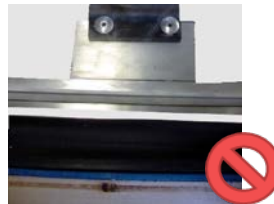
Gasket Too Loose
